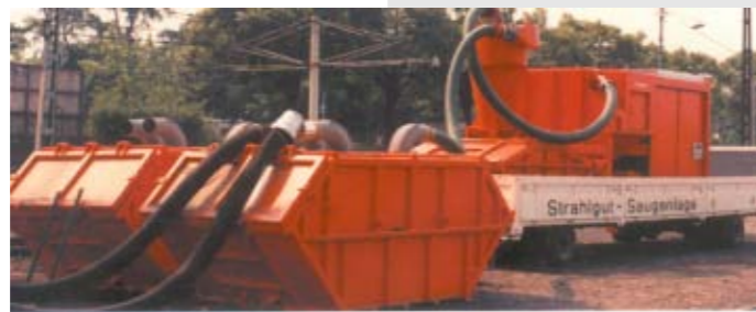
CONTAINERS FOR DISPOSAL OF BLAST MEDIA
