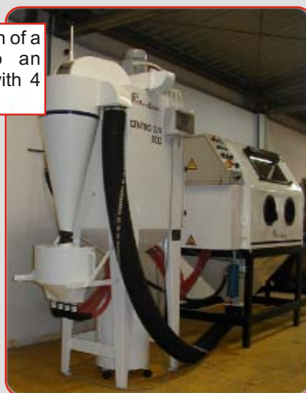
The standard configuration: sandblast cabinet and recycling filter unit CENTRO (here with soundproof fan enclosure)
