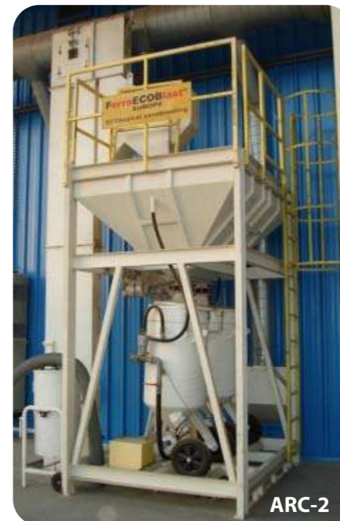
Silo for Abrasive with 2 pressure pots, weighing system and automatic fill-in valves
