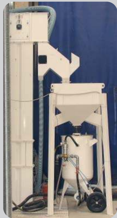
ARC – 1-200 Silo for Abrasive with 1 pressure pot, Elevator & Separator; manuell fill-in valve
