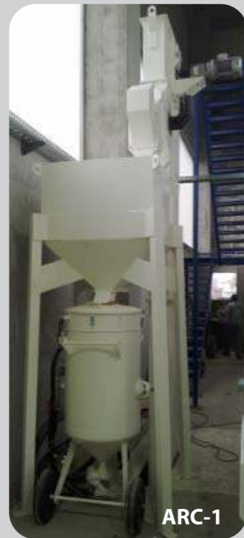
ARC – 1-200 Silo for Abrasive with 1 pressure pot, Elevator & Separator; manuell fill-in valve
