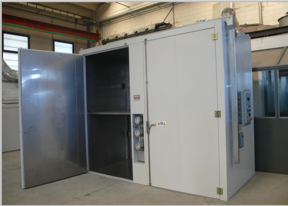
16x Drums Heating Cabinet, up to 150°C, electric operation, ATEX rated.
