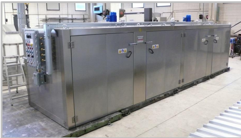
(1/2) FRONT 16x Drums Heating Cabinet, horizontal, divided into 2 x 8 drums independent rooms, up to 150°C, steam operation, Atex rated, AISI304 Stainless steel construction
