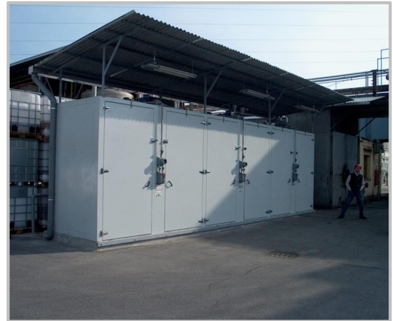
48x Drums Heating Cabinet, horizontal, divided into 3x16 drums independent rooms, up to 150°C, hot oil operation, Atex rated with outdoor installation kit.
