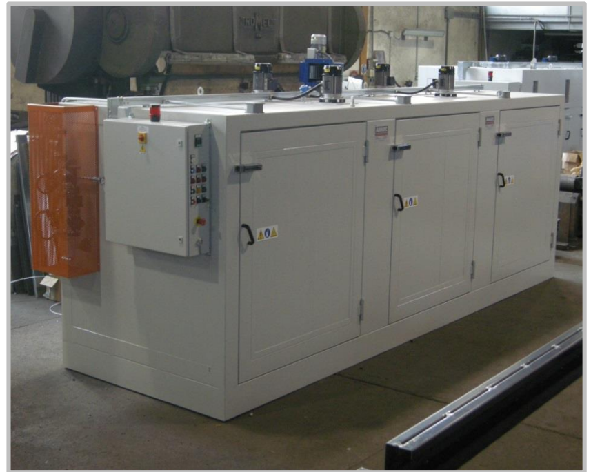
12x Drums Heating Cabinet, horizontal type, up to 100°C, steam operation, with collection sump and exhaust air system.
