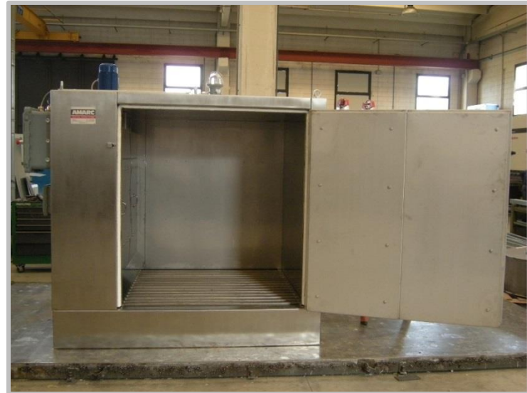
(2/2) 4x Drums Heating Cabinet, up to 150°C, steam operation, ATEX rated, with collection sump , AISI304 stainless steel construction.
