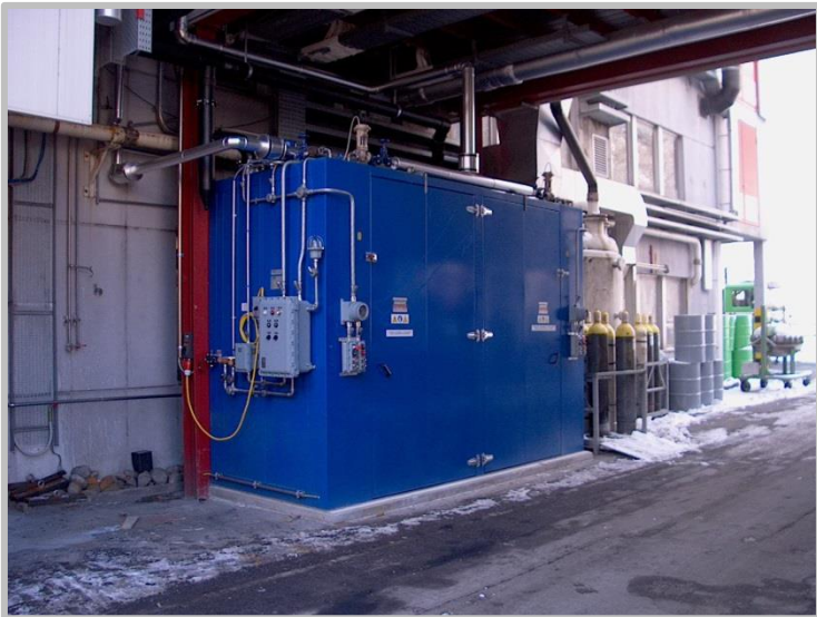
16x Drums Heating Cabinet divided into 2 x 8 drums independent rooms, up to 150°C, hot oil operation, Atex rated.
