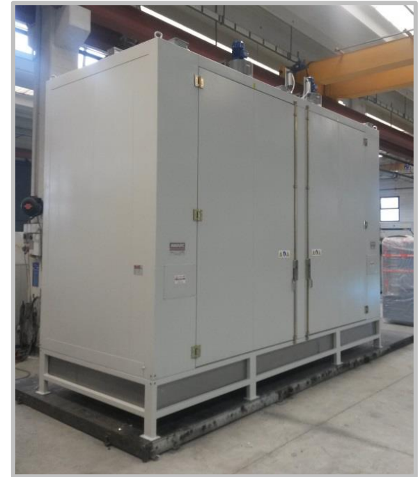
16x Drums Heating Cabinet, divided into 2 x 8 drums room, up to 150°C, electric operation, with base frame with legs and collection sump, internal AISI304 stainless steel panelling, exhaust system with interlocked doors.
