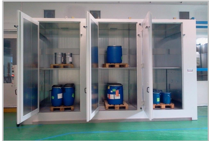
24x Drums Heating Cabinet, divided into 3 x 8 drums rooms, up to 100°C, steam operation, with collection sump.
