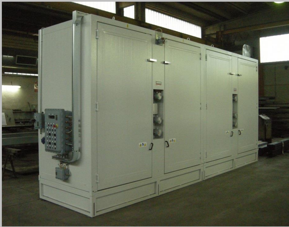
(1\2) FRONT 32x Drums Heating Cabinet, horizontal, divided into 2 x 16 drums independent rooms, up to 150°C, double energy electric +steam operation, Atex rated with collection sump.
