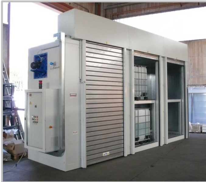
24x Drums Heating Cabinet, up to 80°C, electric operation, with roller shutter doors (and remote control) and collection sump
