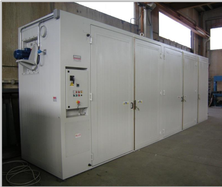
40x Drums Heating Cabinet, up to 90°C, electric operation.
