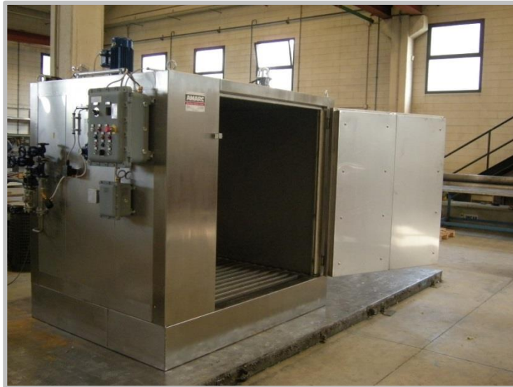
(1/2) 4x Drums Heating Cabinet, up to 150°C, steam operation, ATEX rated, with collection sump , AISI304 stainless steel construction.
