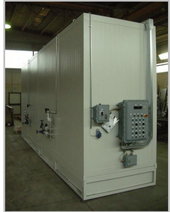
(2\2) BACK 32x Drums Heating Cabinet, horizontal, divided into 2 x 16 drums independent rooms, up to 150°C, double energy electric +steam operation, Atex rated with collection sump
