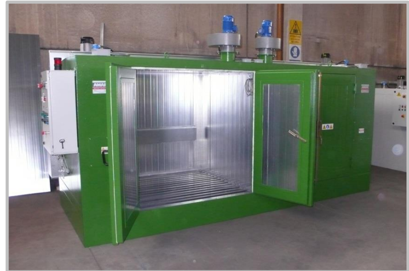
8x Drums Heating Cabinet, EUR compartments, divided into 2 x 4 drums independent rooms, up to 100°C, electric operation, with collection sump and exhaust air system.
